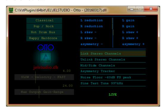
Otto is an automatic amplitude wave-shape equalizer for LIVE or mixing/mastering use.
