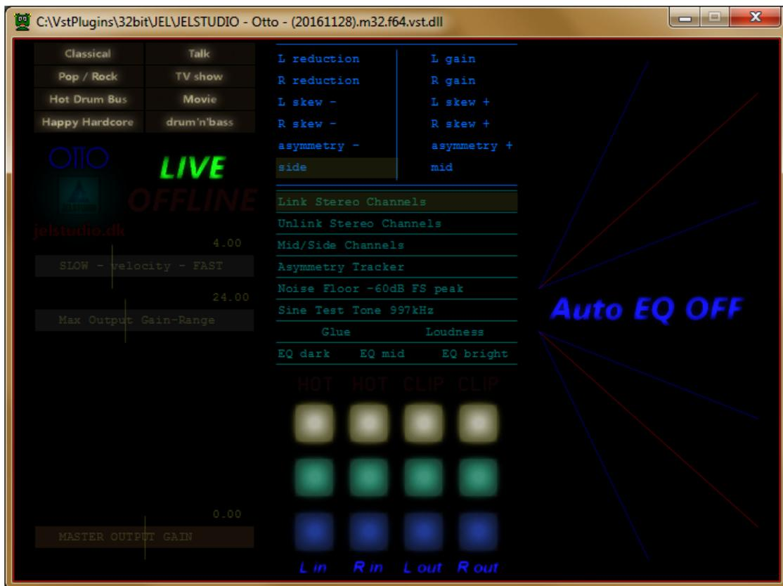
Otto is an automatic amplitude wave-shape equalizer for LIVE or mixing/mastering use.
